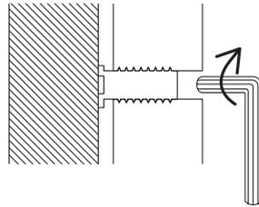
Advice! When mounting on porous wall materials, it might be necessary to fasten pressure distribution washers on the back of the sockets.
